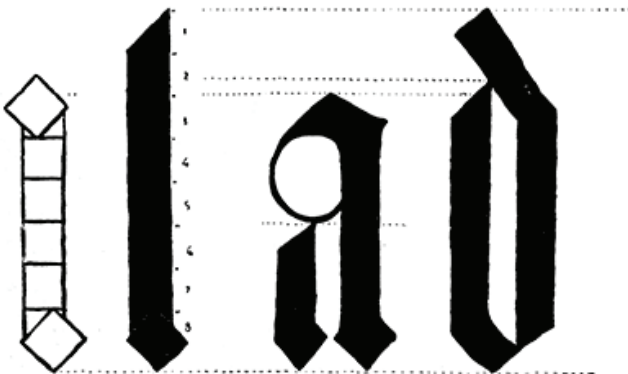
PROPORTIONS OF LOWER-CASE GERMAN TEXT AND METHOD OF DRAWING THE LETTERS (FROM ALBERT DÜRER'S "GEOMETRICA")
